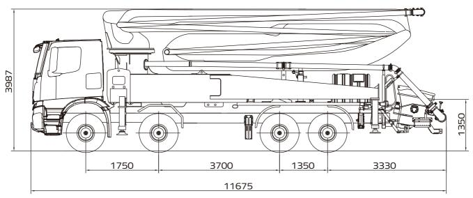
Note: Standard version. Dimensions and weights depend on truck, pump model and equipment. Dimensions in mm. Example based on Mercedes-Benz Arocs 5 3240 8×4. For illustration only. Actual products may vary.
