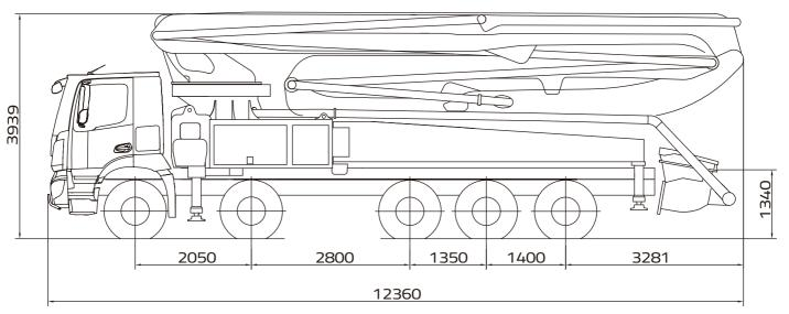
Note: Standard version. Dimensions and weights depend on truck, pump model and equipment. Dimensions in mm. Example based on Mercedes-Benz Arocs 55151.
